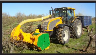
The SERRAT Biomass recovery mulcher consists in a pick-up rotor which lifts up the pruning of fruit trees, vineyard and branches in a second rotor to mulch it. It can be operated by tractors from 150 to 170 HP and 180 to 250 HP with power take off on the front lift.
