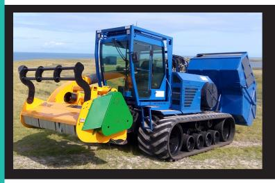
Biosylva mulcher, in just one operation and with the usual speed is able to cut and launch the grass and branches, up to 10 cm of diameter, to a deposit to remove them from the ground.
