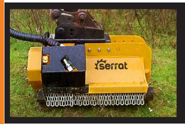
Adaptable for excavators and special carriers having a weight between 6 and 15 t.
