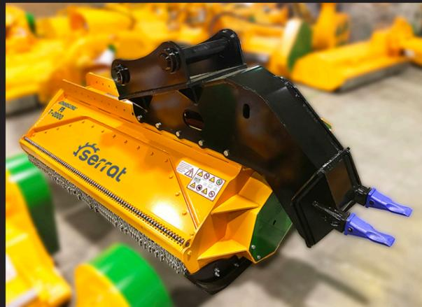
Adaptable for excavators and special carriers having a weight between 25 and 50 t.
