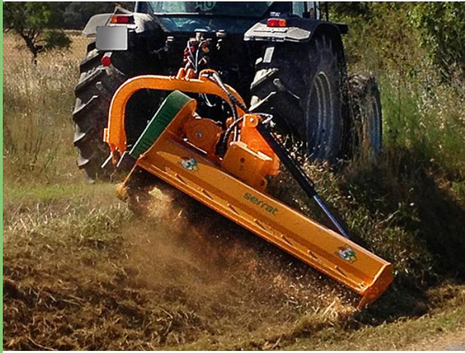
Offset Mulcher of high range, polyvalent, for works in agricultural margins, banks, highways, channels, roads and others clearings of public works for tractor between 70 - 120 HP. It incorporates safety system thanks to a valve positioned in the cylinder of elevation of the arm. It has a rear hood with two positions. Angulation +90° / -65°. Rotor POLSER of 450 mm of diameter with hammer of high edge.
