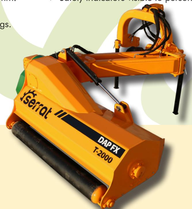
Offset mulcher of high range with forestry rotor, for works in agricultural margins, banks, highways, channels, roads and others clearings of public works for tractors between 120-180 CV. It incorporates safety system thanks to a valve positioned in the cylinder of elevation of the arm.
