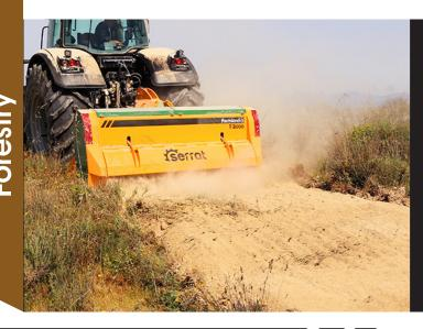
Soil preparation machine up to a depth of 30 cm, for tractors between 130 - 150 HP. Transforms forest land, with stumps and rocks, in land for cultivation avoiding accidents in later processes.
