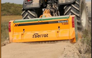
Soil preparation machine up to a depth of 50 cm, for tractors between 250 - 500 HP. Transforms forest land, with stumps and rocks, in land for cultivation avoiding accidents in later processes.
