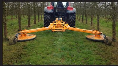
Double mechanical driven swing arms mower conceived to mow around trees, under fences, posts, crash barrier, vineyards, trees, etc. without any damage. Allowing in a single work process to clean two lines of plantation in an average speed of 3 km/hour. We work with a width of 6,30 meters with regard to the axis of the tractor (3,15 m in each sides).
