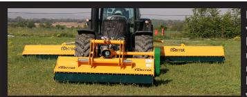
Heavy-duty high body mulcher conceived for very large farms and agricultural contractors. Robust machine designed for very intensive mulching, intended for mulching grass in park maintenance, straw, maize stalks, and on fallow land. Composition for big tractors reaching a working width of 10 meters with a front machine
