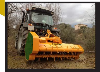
Mulcher with double hydraulic feeder, adapted to cut up residues up to 6-8 cm of diameter in olive trees, citrus fruits, almond trees, walnuts, etc; with interchangeable counter-knives to set the grain size, for tractors between 70 and 120 HP.
