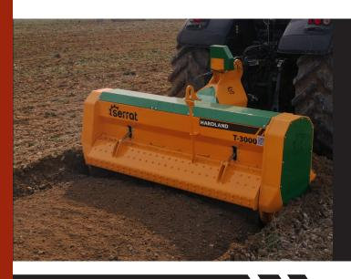
Soil preparation machine up to a depth of 500 mm, for tractors between 350 - 650 HP. Transforms forest land, with stumps and rocks, in land for cultivation avoiding accidents in later processes.
