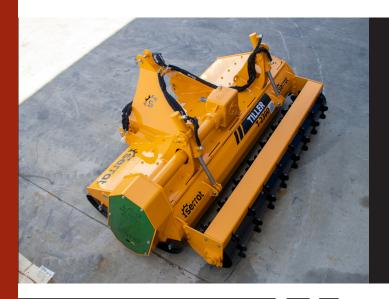
Soil preparation machine up to a depth of 180 mm, for tractors between 100 - 150 HP. Transforms forest land, with stumps and rocks, in land for cultivation avoiding accidents in later processes.
