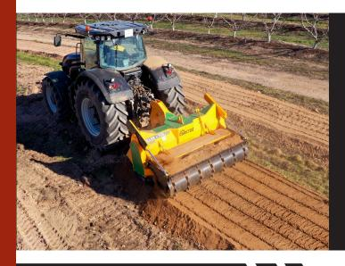
Soil preparation machine up to a depth of 500 mm, for tractors between 300 - 600 HP. Transforms forest land, with stumps and rocks, in land for cultivation avoiding accidents in later processes.
