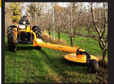
Mechanical driven swing arm mower can be used to mow around trees, posts, crash barrier, etc. Without any damage.
