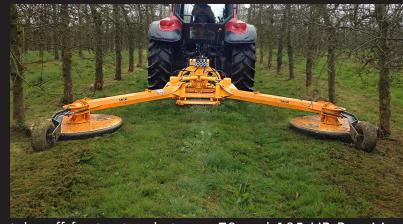
Double mechanical driven swing arms mower conceived to mow around trees, under fences, posts, crash barrier, vineyards, trees, etc. without any damage. Allowing in a single work process to clean two lines of plantation in an average speed of 3 km/h. We work with a width of 6,30 m with regard to the axis of the tractor (3,15 m in each sides). Mechanical transmission by power
