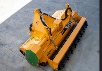
Soil preparation machine up to a depth of 180 mm, for tractors between 100 - 130 HP. Transforms forest land, with stumps and rocks, in land for cultivation avoiding accidents in later processes.
