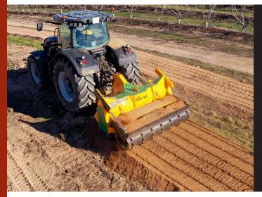
Soil preparation machine up to a depth of 500 mm, for tractors between 300 - 400 HP. Transforms forest land, with stumps and rocks, in land for cultivation avoiding accidents in later processes.
