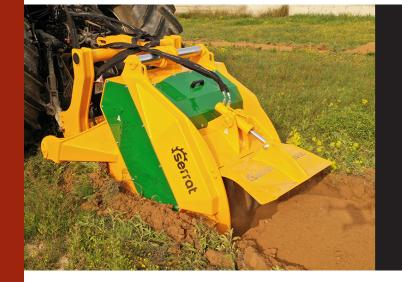
Soil preparation machine up to a depth of 400-500 mm, for tractors between 200 - 350 HP. It mulchs the stumps of old plantations, leaving a soft ground for the next plantation.
