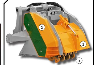
3. Teeth fitted inside the rotor
