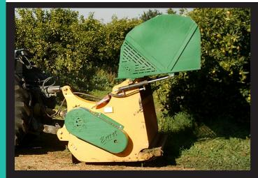
Mulcher for the cut and withdrawal of grass and branches up to 80 mm of diameter.
