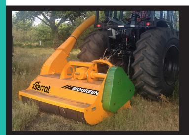
Biogreen mulcher, in just one operation and with the usual speed is able to cut and launch the grass and branches to a deposit to remove them from the ground.
