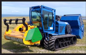
Biosylva mulcher, in just one operation and with the usual speed is able to cut and launch the grass and branches, up to 100 mm of diameter, to a deposit to remove them from the ground.
