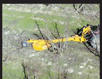
Mechanically operated vertical axis disc for cutting fruit tree trunks. Up to 150-200 mm in diameter.
