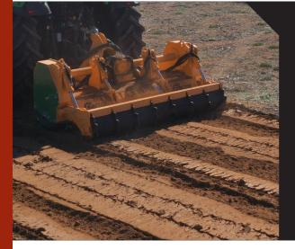
Soil preparation machine up to a depth of 250 mm, for tractors between 80 - 130 HP. Transforms forest land, with stumps and rocks, in land for cultivation avoiding accidents in later processes.
