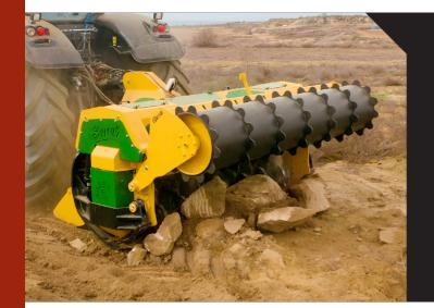
Soil preparation machine up to a depth of 400 mm, for tractors between 400 - 700 HP. Transforms forest land, with stumps and rocks, in land for cultivation avoiding accidents in later processes.
