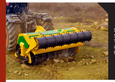
Soil preparation machine up to a depth of 500 mm, for tractors between 400 - 700 HP. Transforms forest land, with stumps and rocks, in land for cultivation avoiding accidents in later processes.
