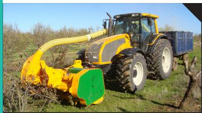
The SERRAT Biomass recovery mulcher consists in a pick-up rotor which lifts up the pruning of fruit trees, vineyard and branches in a second rotor to mulch it. It can be operated by tractors from 150 to 250 HP and 200 to 250 HP with power take off on the front lift.
