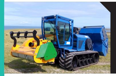
Biosylva mulcher, in just one operation and with the usual speed is able to cut and launch the grass and branches, up to 100 mm of diameter, to a deposit to remove them from the ground.
