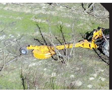
Mechanically operated vertical axis disc for cutting fruit tree trunks. Up to 150-200 mm in diameter.
